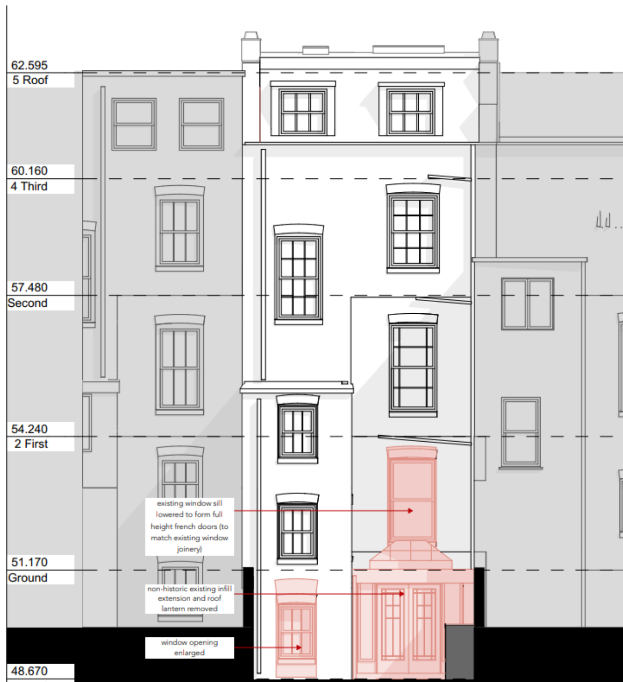
Drawing 1: Rear Elevation – Demolition
